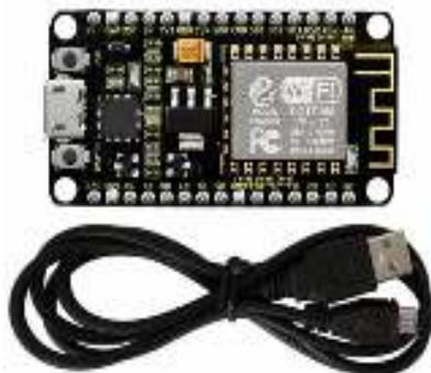
Gambar 2 NodeMCU
