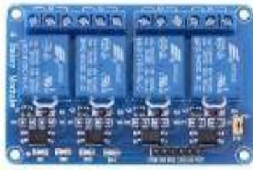
Gambar 2.5 Relay Module
