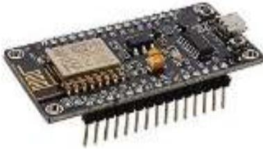
Gambar 2.1 NodeMCU
